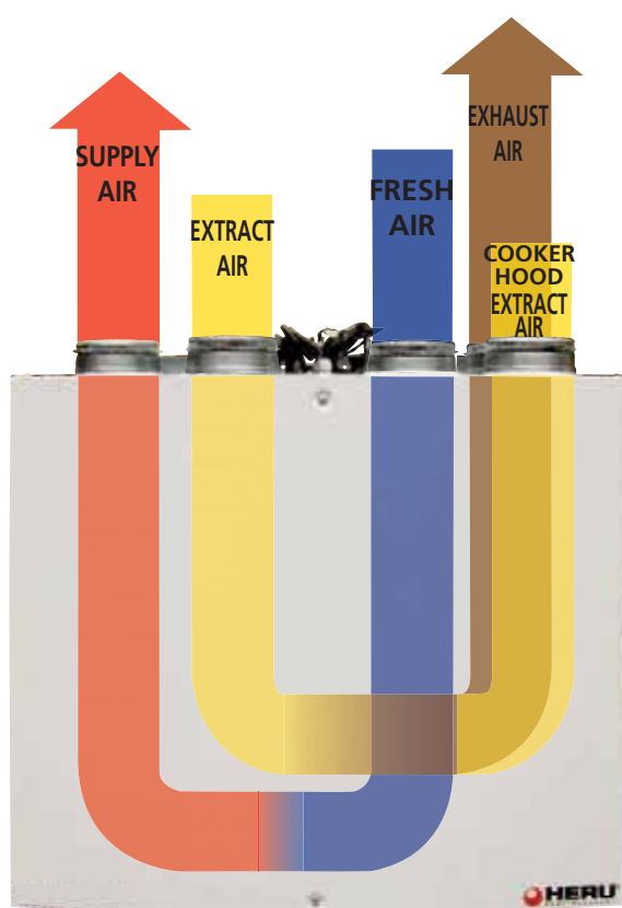
LEFT HANDING APPLICATION: HERU®70 T, 100 T EC, 160 T EC (WITH OR WITHOUT COOKER HOOD CON.). HERU®200 T EC, 250 T, 250 T EC (EXCEPT COOKER HOOD CON.).
